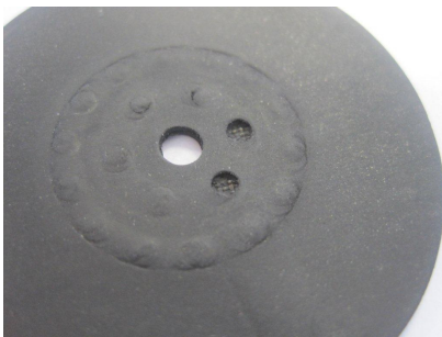
Some examples of damaged diaphragms
