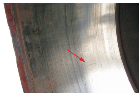
Scorches and temper colours with heat cracks starting to form
