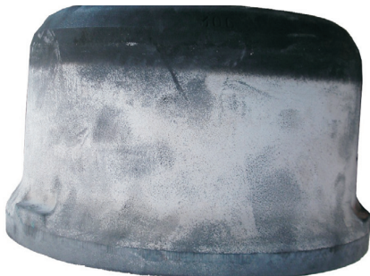
Scorches and temper colours with heat cracks starting to form
