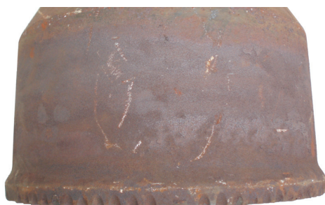
Scorches and temper colours with heat cracks starting to form
