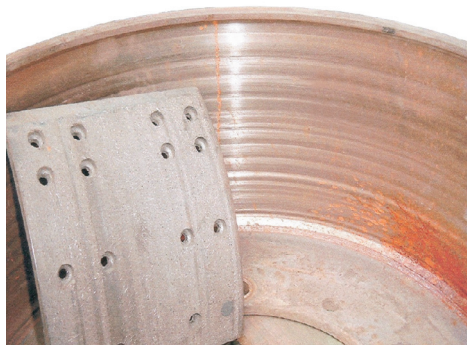
a) Scoring due to coarse dirt
