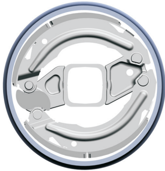
a) Brake drum with radial run-out
