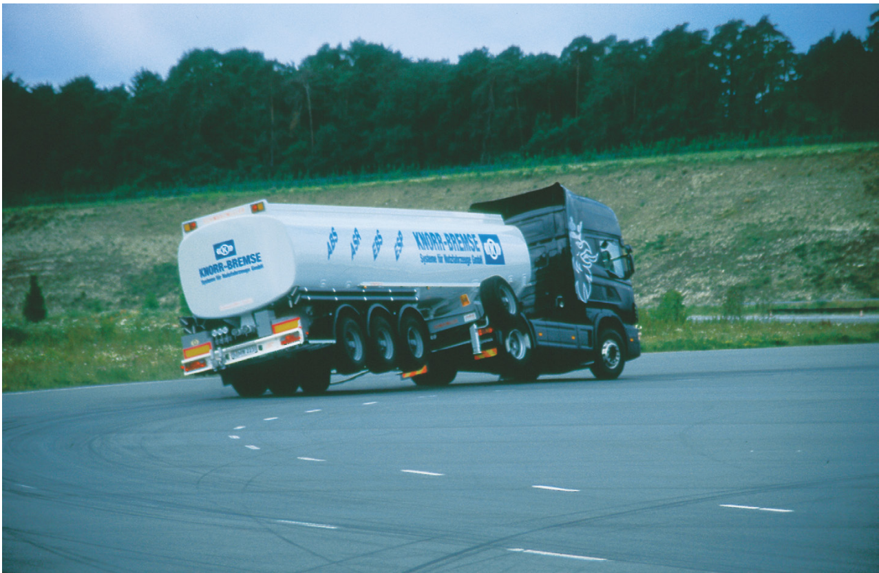
ESP switched off Image supplied by Knorr-Bremse UK
