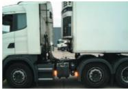
The first stage of the procedure involves the connection of the trailer to the fifth wheel while it is located rearward of the normal
