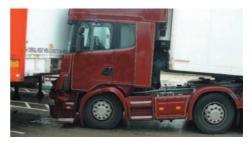
The roll away of a trailer, when the towing unit is correctly parked, is likely to have the same consequences as a complete vehicle or towing unit run away. In many cases the cause of this type of accident is due to bad practice of both the driver who left the trailer without applying the parking brake, and the driver coupling to the trailer, who did not check that the parking brake was applied and subsequently had the accident.
